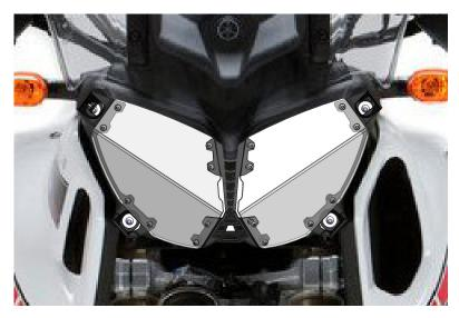
Install headlight guard. !TIP A dab of water on each ball stud will help it fit in place easier with less wear on the rubber grommets.
