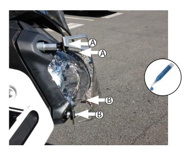
Apply a small drop of loctite to the threads of each ball stud. Insert longer 40mm extension ball studs into upper two positions(A). Insert shorter 25mm ball studs into lower positions(B). Tighten to 6.5Nm.
