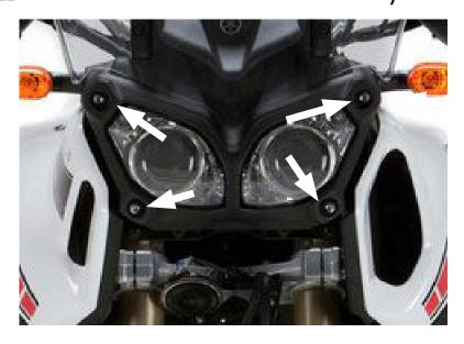
Use 5mm allen and remove four screws shown.
